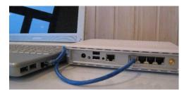
Press the Restore button (the recessed black button on the back) on the router and turn on the router (connect the power).
