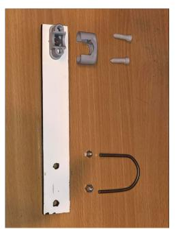
Create 4 distance holders as per picture on the left. The Trespa / Plexiglas strips are 20x2 cm each and are 5mm thick.
